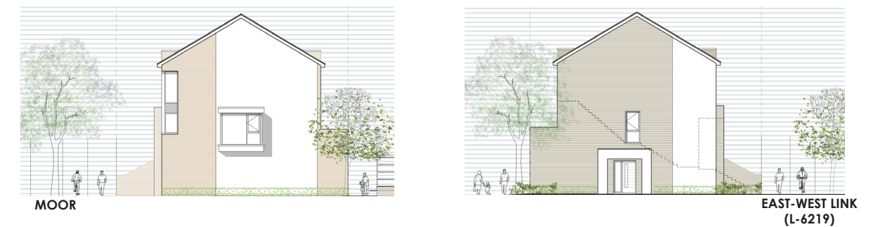
Figure 78. Proposed design for gable elevations of duplex buildings showing prominent entrance to ground floor units and windows of duplex unit ensuring aesthetic streetscapes and passive surveillance of public realm and communal areas adjacent. Source: MCORM, 2022.
